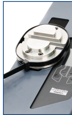
Cable Tie fixture (part no. 432-653) (See DS-1162)
