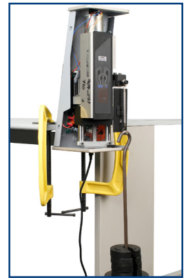
Calibration rig for simple verification of load reading (See DS-1166)
